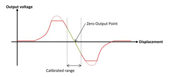
Transducer range will be ±X.Xmm around the Zero Output Point depending on which model is used.
