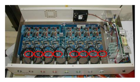
As indicated by GDS move the required channels jumper in the correct position.
