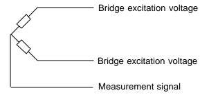
**Linear Potentiometers** - These are half bridge transducers and work with a 4.8kHz carrier-frequency amplifier module.
