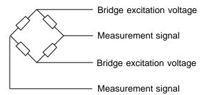
**Load Cells** - These are full bridge transducers and work with a 4.8kHz carrier-frequency amplifier module.
