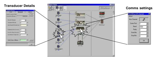
Assuming the hardware is connected to the system correctly, clicking on the "EYE" icon will bring up the transducer details. It is important to enter the correct details in the ADVANCED tab such as Transducer Full Scale, Decimal Places and Transducer Upper Limit. The calibration tab is also important, where either a full calibration may be performed, or the transducer sensitivity is entered.
