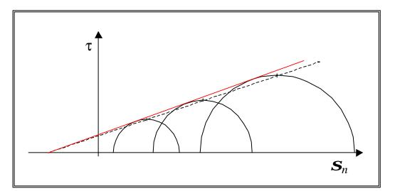
This line is called the MODIFIED FAILURE ENVELOPE. Let the slope be q and the intercept be **k**.
