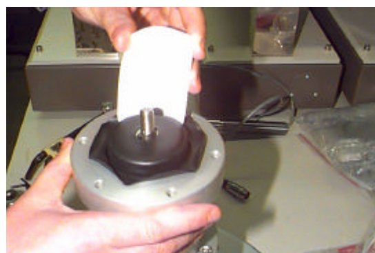
Photographs 1a and 1b above shows the top bellofram being changed.
