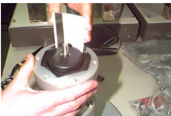
Photographs 1a and 1b above shows the top bellofram being changed.
